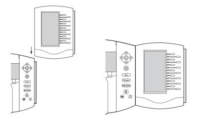
(3) To connect up to three Expansion Modules together, repeat steps ① and ②.
